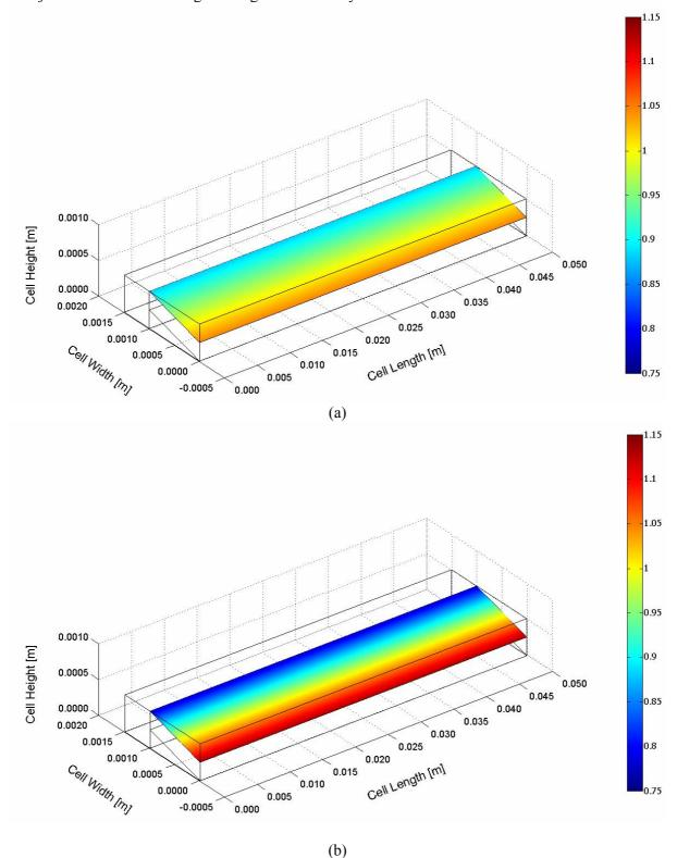
Figure 6. Local current density distribution at the cathode catalyst layer for two different nominal current densities: (a) 0.2 A/cm<sup>2</sup> and (b) 0.4 A/cm<sup>2</sup>
