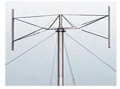
Figure 1. H-Darrieus wind rotor
