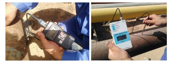
Figure 2. Ultrasonic thickness gauge.
