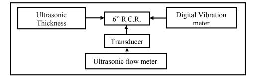
Figure 5. Experimental work block diagram.
