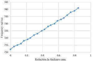
Figure 8. The relationship between the reduction in the thickness of the pipe and the value of its vibration is as positive.
