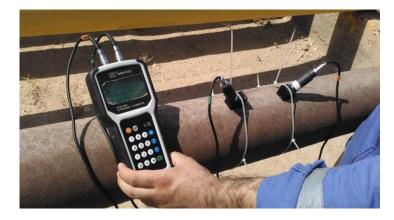
Figure 4. Ultrasonic Flow-meter.
