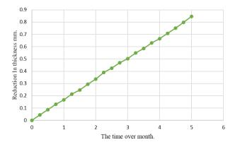
Figure 9. The value of the pipe thickness reduction with the time.
