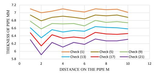
Figure 6. The condition in which the metal is corroded due to the flow over time (every one year).
