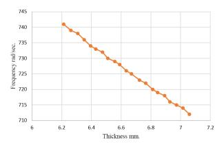
Figure 7. The reduction in the thickness of the pipe increases the value of frequency.
