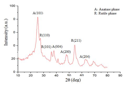
Figure 2. X-ray diffraction of prepared TiO<sub>2</sub> nano-particles.
