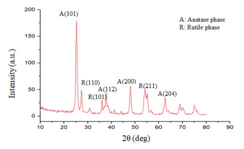
Figure 3. X-ray diffraction pattern of TiO<sub>2</sub> powder at 500 °C.
