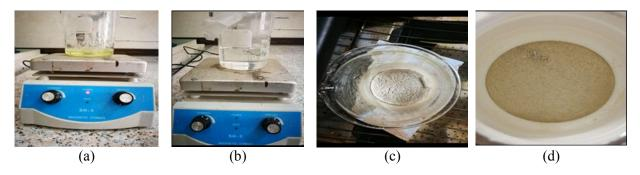
Figure 1. Preparation steps of TiO<sub>2</sub> nanoparticle: (a) TiCl<sub>4</sub> solution added to ethanol, (b) Distilled water was added, (c) The final sol–gel solution dried at 50 °C for 16 h, (d) after treated it at 500 °C to form TiO<sub>2</sub> powder.
