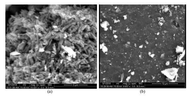
Figure 5. SEM images of TiO<sub>2</sub> powder Annealing at 500 C° [A] 5µm, [B] 10µm.
