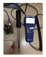
Figure 2. Calibration of DHT22 sensor.
