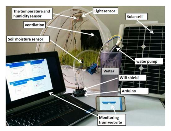
Figure 3. Smart greenhouse prototype.
