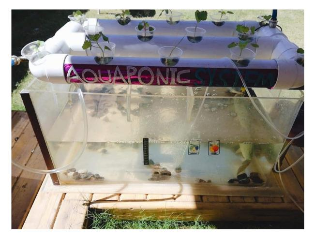
Figure 3. Setup of the proposing system.
