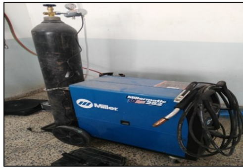
Figure 1. The inert gas arc welding machine.
