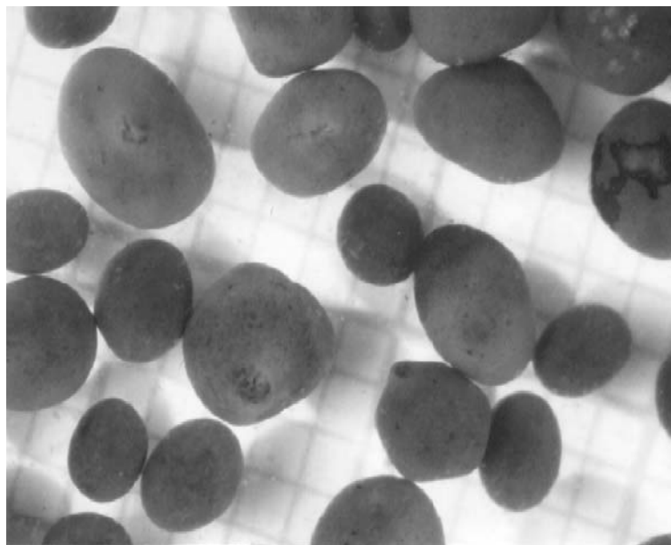
Figure 2. Anaerobic sludge granules from a UASB reactor Hulshoff [7]
