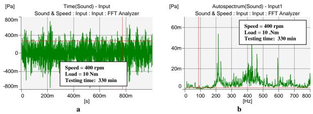
Figure 11. Sound pressure level spectra: (a) time history (g4), 3.0 x 0.5 x 40 mm; and (b) frequency domain (g4), 3.0 x 0.5 x 40 mm
