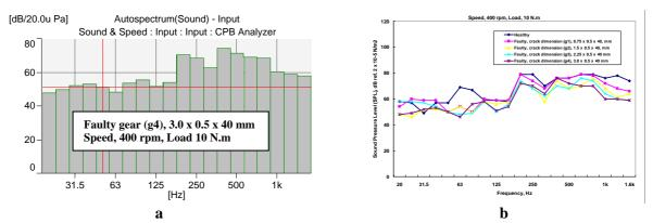
Figure 8. 1/3-Octave sound pressure level spectra: (a) 1/3-octave sound pressure level; and (b) 1/3-octave sound pressure level
