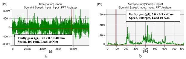
Figure 7. Sound pressure level spectra: (a) time history of sound pressure level; and (b) frequency domain of sound pressure level
