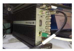
Figure 2. Bruel & Kjaer (B&K) portable and multichannel PULSE
