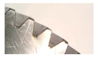
Figure 4. Gear tooth crack
