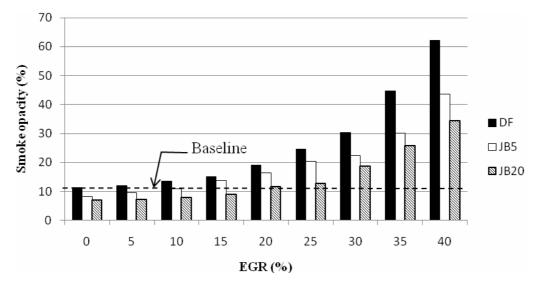
Figure 11. Variation of smoke opacity with various EGR rates
