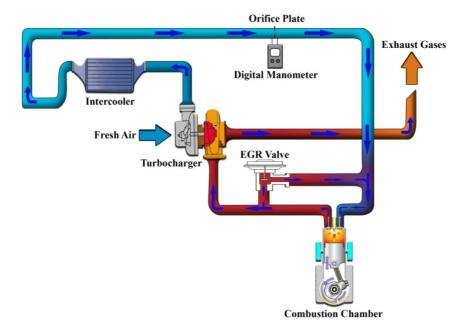
Figure 1. A schematic diagram of EGR system
