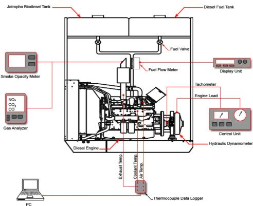
Figure 2. A schematic diagram of experimental setup
