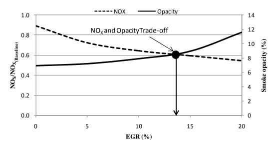
Figure 13. The optimum trade-off between NO<sub>x</sub> and smoke opacity for different EGR rates with JB20
