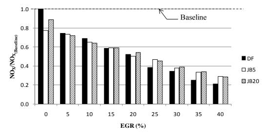
Figure 10. Variation of NO<sub>X</sub> emission with various EGR rates
