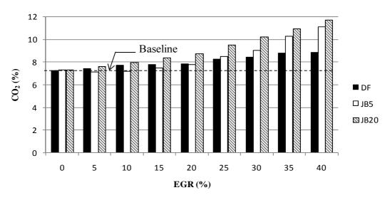
Figure 9. Variation of CO<sub>2</sub> emission with various EGR rates
