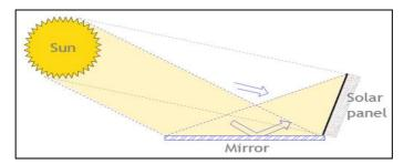
Figure 10. Use of reflecting media with solar panel
