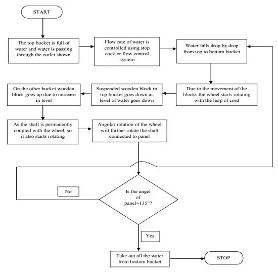
Figure 9. The flow chart of working norm of proposed solar tracker
