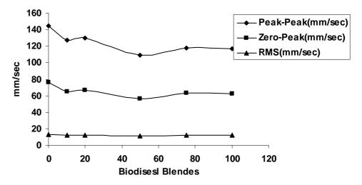
Figure 10. Effect of blend ratio on vibrations (axial)
