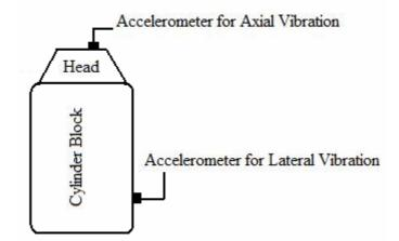
Figure 1. Positions of accelerometer
