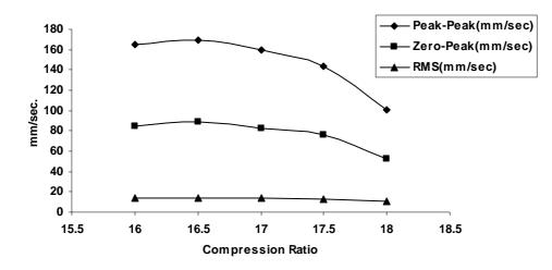
Figure 6. Effect of compression ratio on vibrations (axial)
