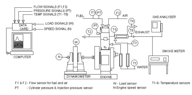
Figure 2. Engine test setup
