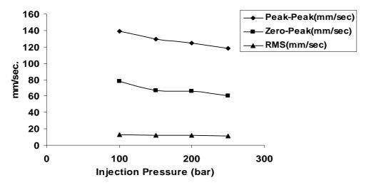
Figure 8. Effect of Injection pressure on vibrations (axial)
