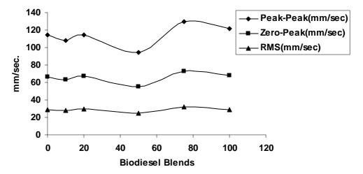
Figure 9. Effect of blend ratio on vibrations (lateral)
