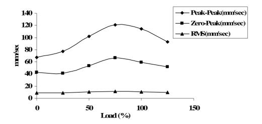
Figure 4. Effect of brake load on vibrations (axial)
