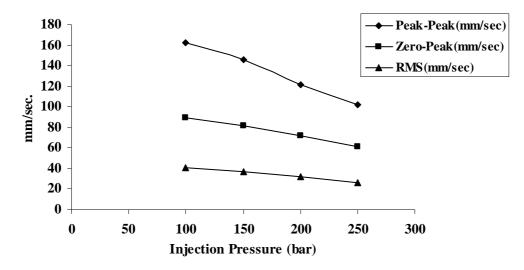
Figure 7. Effect of Injection pressure on vibrations (lateral)
