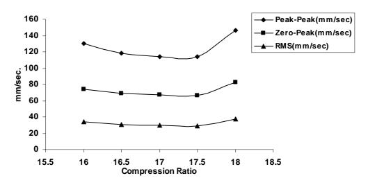
Figure 5. Effect of compression ratio on vibrations (lateral)
