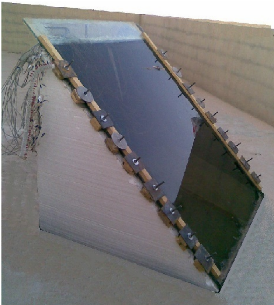
Figure1. The experimental integrated collector storage system
