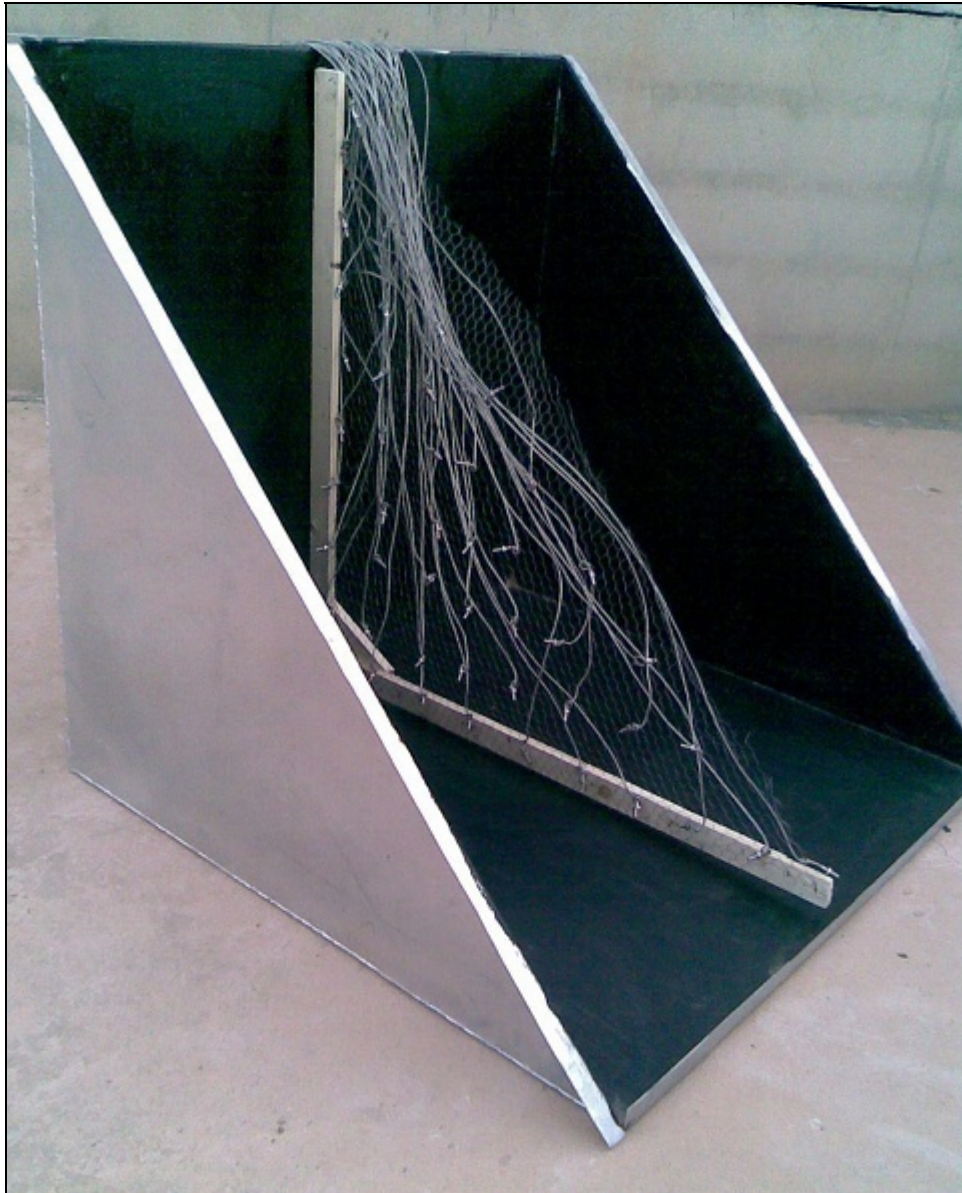
Figure 2. Thermocouples distribution inside the tank
