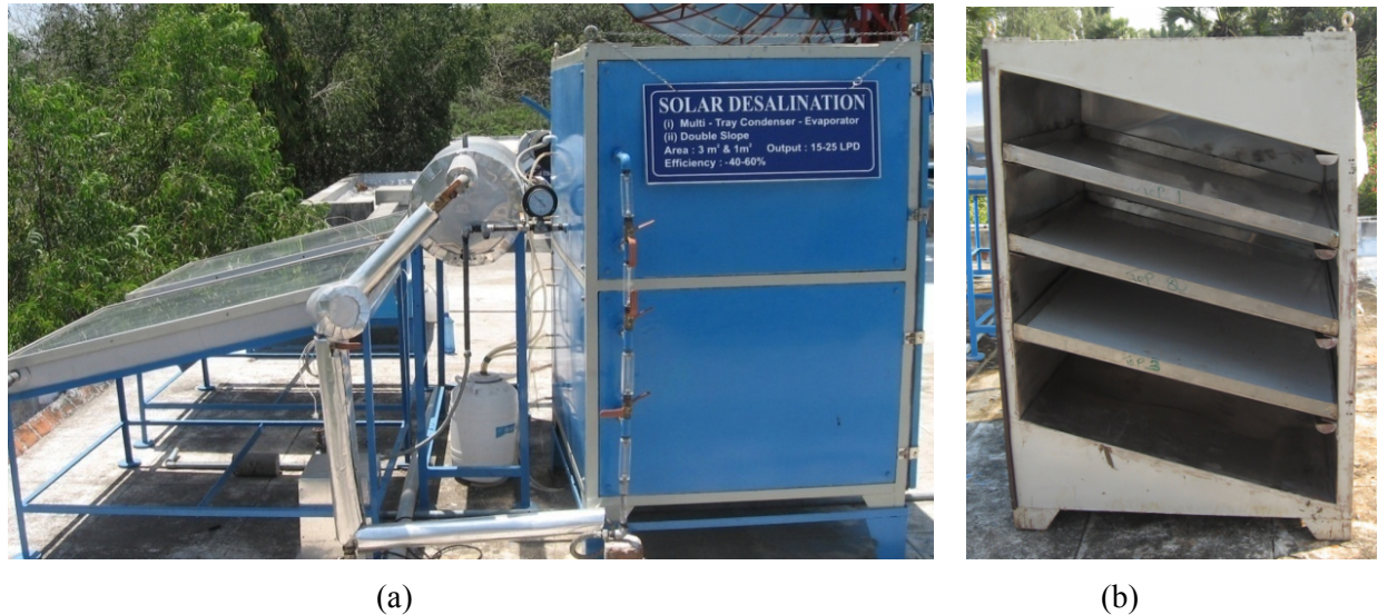
Figure 2. Multi-stage evacuated solar desalination system; (a) Experimental Set up, (b) Inside View of the system
