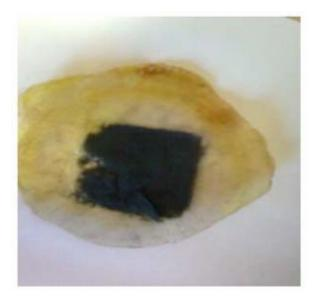
Figure 1. Composite membrane (Nafion/TiO<sub>2)</sub>
