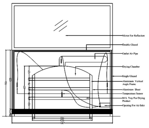
Figure 1. Front view of solar dryer with mirror booster
