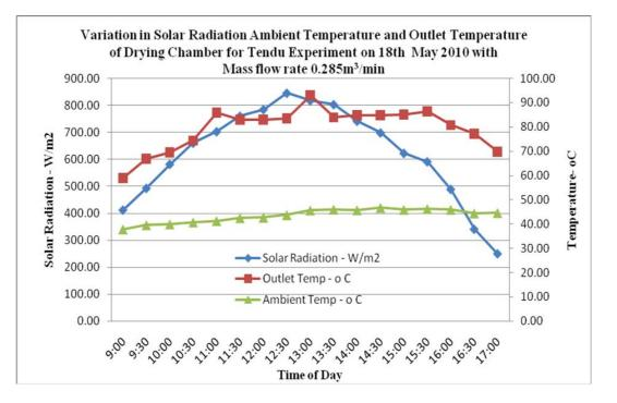
Figure 2. Variations of solar radiation, ambient temperature and drying air temperature at the outlet of the drying chamber with time on 18<sup>th</sup> May 2010 during solar drying of Tendu leaf with mass flow rate of 0.285 m<sup>3</sup>/min
