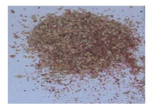
Figure 1. Crushed and ground maize cobs
