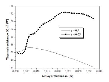
Figure 8. Thermal resistance as a function of the air cavity thickness, case of a cinderblock
