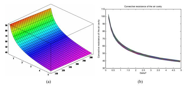
Figure 4. (a) variation of  $R_{CV}$  as function of T and  $\Delta\theta$ ; (b)  $R_{CV}$  as a function of  $\Delta\theta$  for T ranging from 0 to 60 ° C
