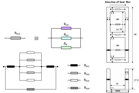
Figure 1. Dimensions (in centimeters) and equivalent circuit of a cinderblock
