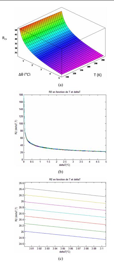
Figure 2. (a) variation of  $R_{CV}$  as function of T and  $\Delta\theta$ ; (b)  $R_{CV}$  as a function of  $\Delta\theta$  for T ranging from 0 to 60 ° C; (c) zoom
