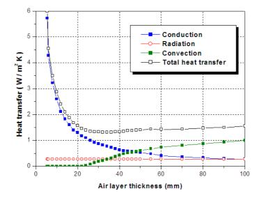
Figure 6. Estimated heat transfer in a closed air cavity bounded by a reflective material at one face  $\epsilon = 0.05$
