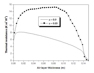
Figure 7. Thermal resistance as a function of the air cavity thickness, case of a cinderblock
