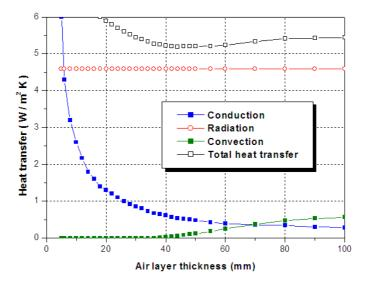
Figure 5. Estimated heat transfer in a closed air cavity bounded by ordinary materials  $\varepsilon = 0.9$
