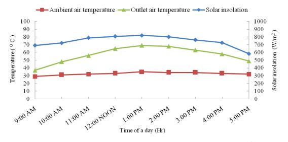
Figure 7. Hourly variations of solar radiation, ambient air and outlet air temperatures (1<sup>st</sup> February 2011)
