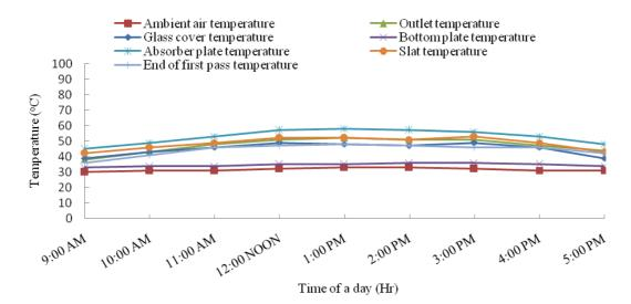
Figure 6. Hourly temperature variation of double pass hybrid (PV/T) air heater with respect to time of the day
