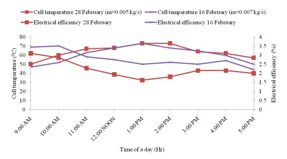
Figure 9. Hourly variation of cell temperature and electrical efficiency for the month of February, 2011
