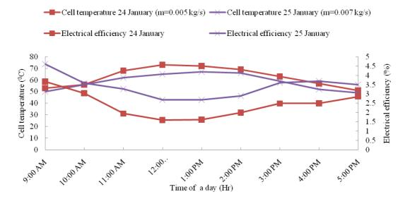
Figure 8. Hourly variation of cell temperature and electrical efficiency for the month of January, 2011
