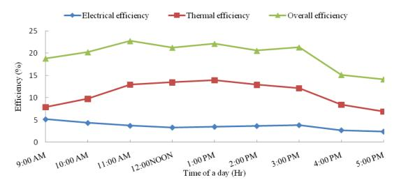
Figure 11. Variation of electrical, thermal and overall efficiencies (22 February 2011)
