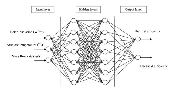
Figure 5. Architecture of ANN used for the performance prediction
