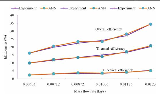
Figure 13. Comparison of electrical, thermal, and overall efficiencies (Experimental and ANN predicted)
