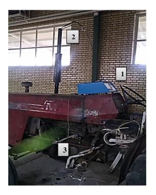
Figure 1. Details of specific device (1. Gas analyzer, 2. Gas inlet, 3. Oil temperature sensor)
