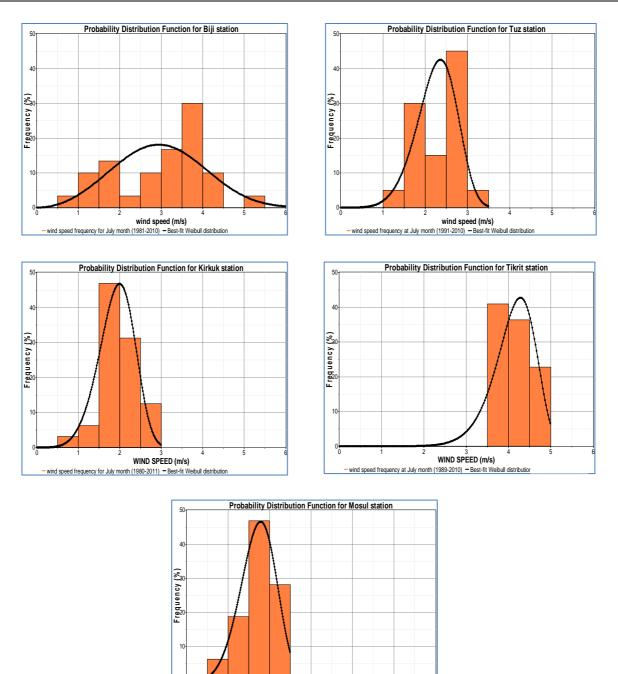
Figure 5. Histogram of the wind speed distributions simulated by Weibull function during July for the sites Biji, Tuz,Tikrit, Kirkuk, Mosul
