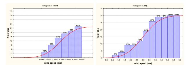
Figure 6. Cumulative wind speed frequency distribution of Biji and Tikrit stations
