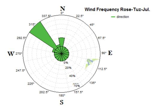
Figure 3. Wind direction frequency (wind rose) at July month for Tuz station (1991-2010)
