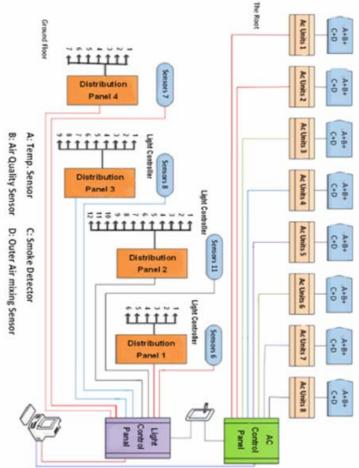
Figure 1. Schematic diagram of the BMS in a typical building
