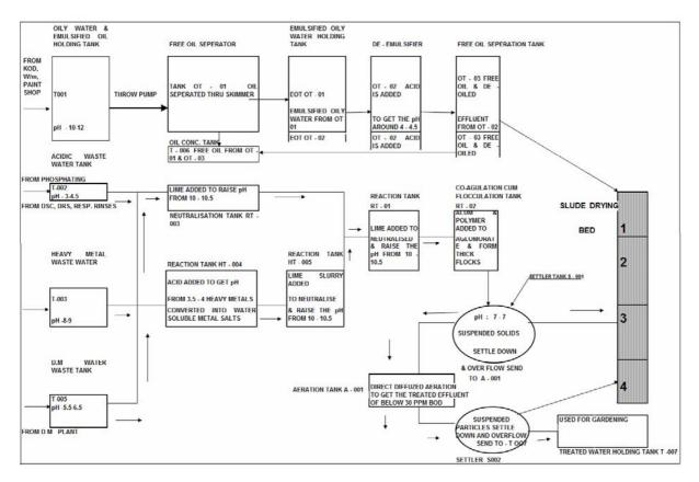
Figure 1. Flow diagram of effluent treatment plant
