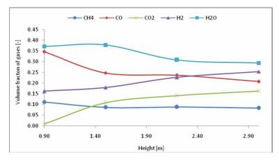
Figure 10. Gas volume fraction along the height of the reactor
