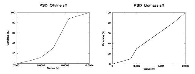
Figure 3. Particle size distribution of the bed material and biomass
