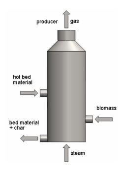
Figure 2. fModel of gasification reactor
