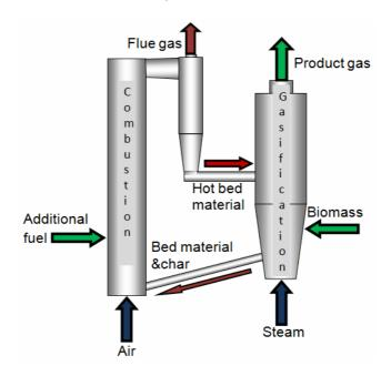
Figure 1. Principle of dual fluidized bed-gasification process
