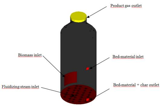
Figure 4. Pressure and flow boundary condition of the model
