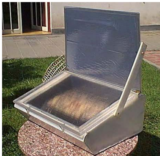
Figure 2. Physical model of the solar oven
