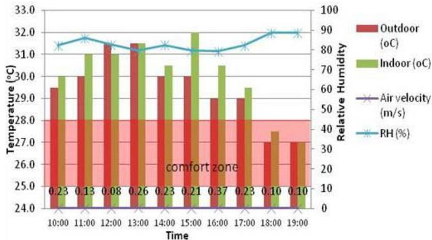
Figure 4. Outdoor, Indoor temperature, air velocity and relative humidity measurement data
