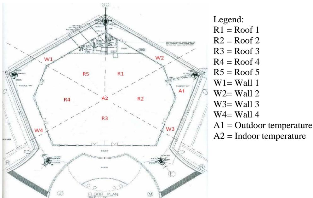
Figure 2. The location of surface, indoor and outdoor temperature measurement
