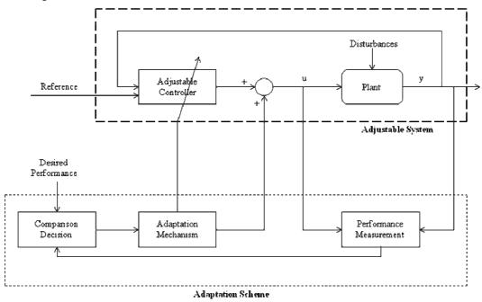
Figure 1. Basic configuration of adaptive control system [38]
