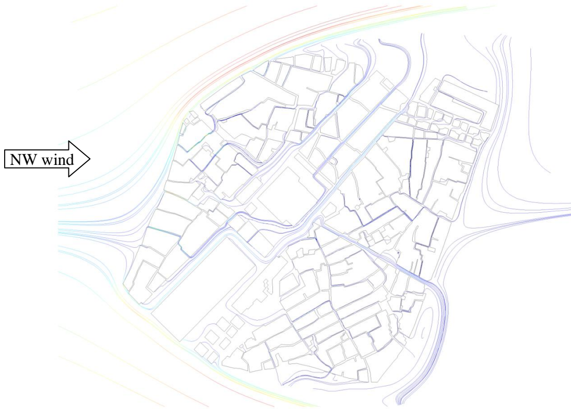
Figure 3. Plan view of streamlines showing flow direction and wind speeds in the historic city centre.
