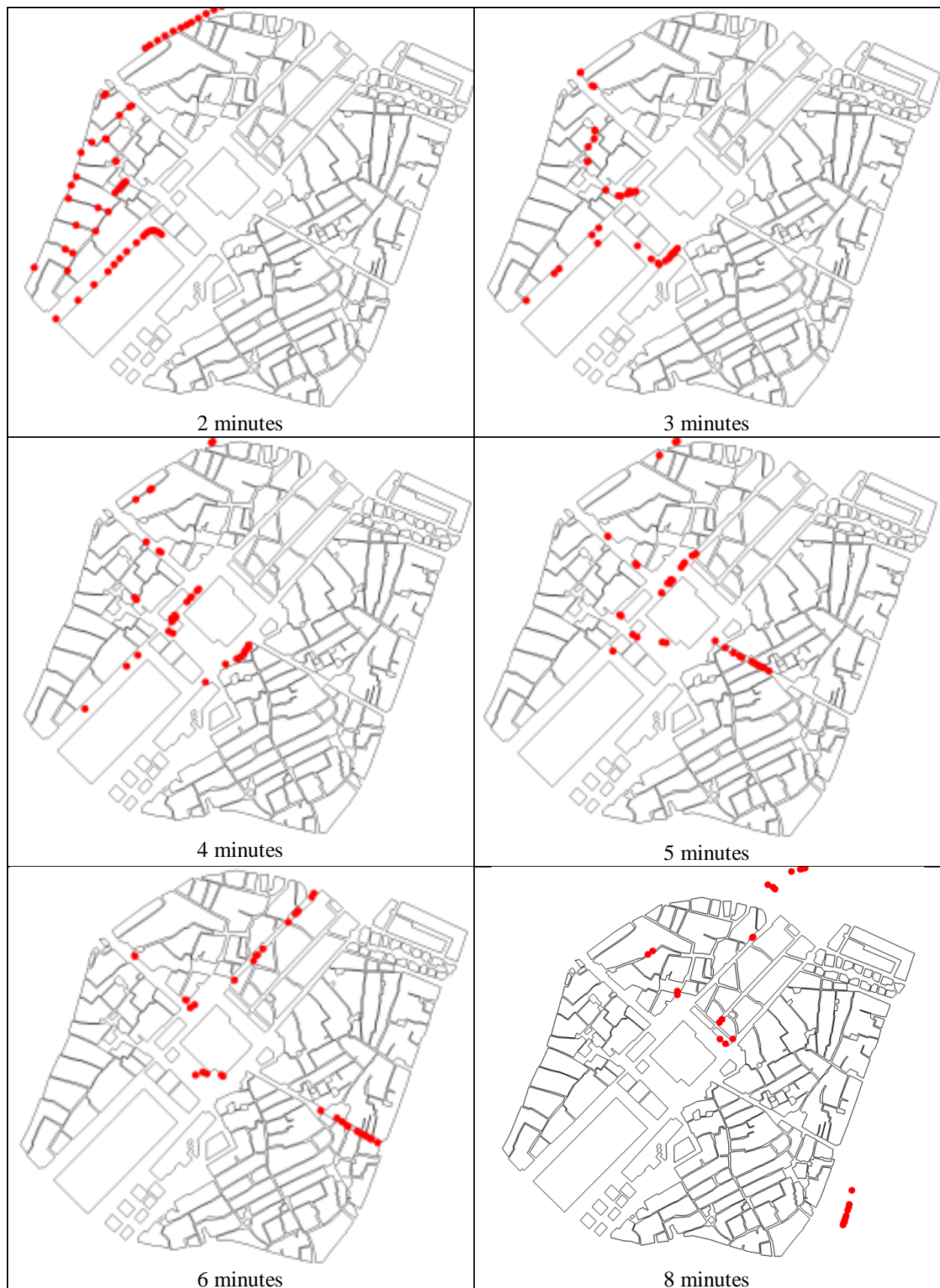
Figure 5. Visualizations of the dust particles in the wind through the city. The source was an instantaneous release of a neutrally buoyant tracer dust particles at ground level in the historic city centre. The frames show relative tracer concentrations at 2, 3, 4, 5, 6 and 8 minutes after release.
