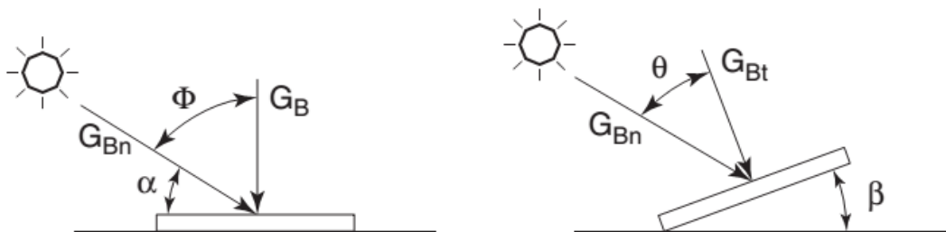
Figure 4. Beam radiation on horizontal and tilted surfaces [6]
