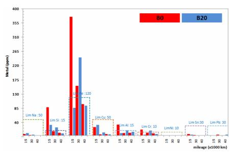
Figure 8.Wear metals analysis of the vehicle B.
