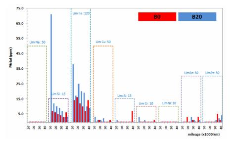
Figure 9. Wear metals analysis of the vehicle C.
