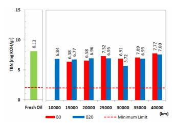
Figure 6. TBN for the vehicle C.
