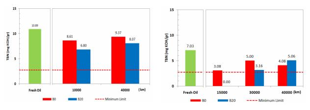
Figure 4. TBN for the vehicle A.
