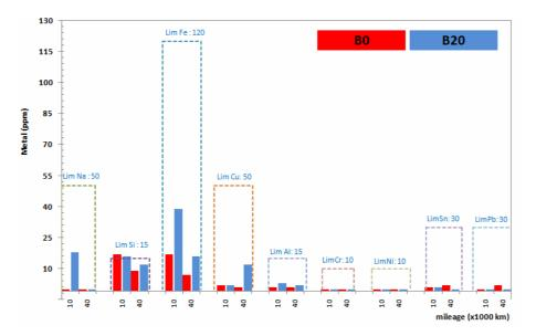
Figure 7. Wear metals analysis of the vehicle A.
