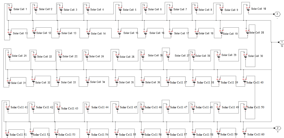
Figure 6. Sixty series cells of a single SOLIMPEKS PV module.
