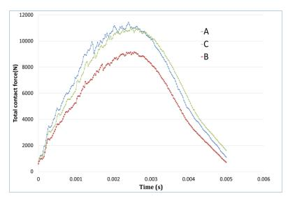
Figure 9. Numerical the total force-time histories at impact energy 35 J (A  $[90_2, -45_2, 0_2, 45_2]_{2s}$ , B  $[0_2, 45_2, -45_2, 90_2]_{2s}$ , C  $[45_2, 0_2, 90_2, -45_2]_{2s}$ ).
