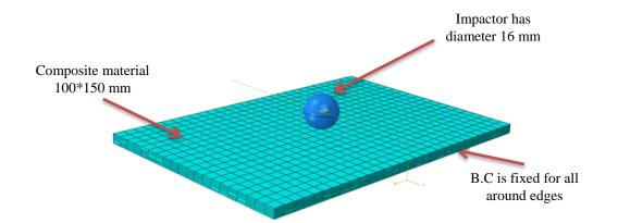
Figure 4. Model of impact, in numerical model three composite with different stacking sequences A  $[90_2, -45_2, 0_2, 45_2]_{2s}$ , B  $[0_2, 45_2, -45_2, 90_2]_{2s}$  and C  $[45_2, 0_2, 90_2, -45_2]_{2s}$ .
