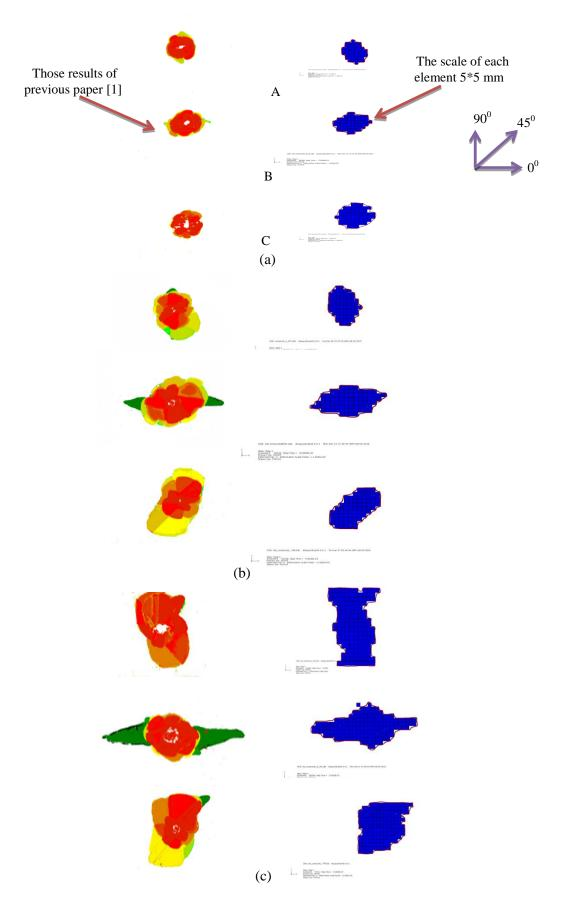
Figure 5. Numerical models of the total delamination compared with experimental results (a) impact energy 15 J, (b) impact energy 25J and (c) impact energy 35J. (( $\mathbf{A}$  [90<sub>2</sub>, -45<sub>2</sub>, 0<sub>2</sub>, 45<sub>2</sub>]<sub>2s</sub>), ( $\mathbf{B}$  [0<sub>2</sub>, 45<sub>2</sub>, -45<sub>2</sub>, 90<sub>2</sub>]<sub>2s</sub>), ( $\mathbf{C}$  [45<sub>2</sub>, 0<sub>2</sub>, 90<sub>2</sub>, -45<sub>2</sub>]<sub>2s</sub>)).
