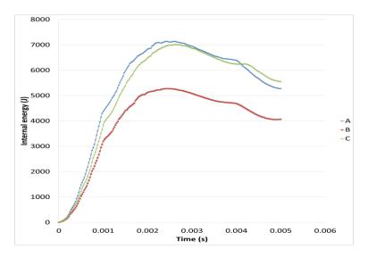
Figure 8. Numerical the internal energy-time histories at impact energy 35 J (A  $[90_2, -45_2, 0_2, 45_2]_{28}$ , B  $[0_2, 45_2, -45_2, 90_2]_{28}$ , C  $[45_2, 0_2, 90_2, -45_2]_{28}$ ).
