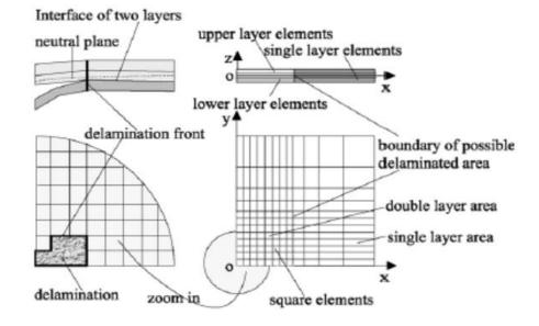
Figure 2. The FEM delamination model [23].
