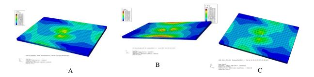
Figure 11. Stress contours for composite plate at impact energy 35 J for carbon fiber/epoxy (A [90<sub>2</sub>, -45<sub>2</sub>, 0<sub>2</sub>, 45<sub>2</sub>]<sub>2s</sub>), (B [0<sub>2</sub>, 45<sub>2</sub>, -45<sub>2</sub>, 90<sub>2</sub>]<sub>2s</sub>), (c) (C [45<sub>2</sub>, 0<sub>2</sub>, 90<sub>2</sub>, -45<sub>2</sub>]<sub>2s</sub>).
