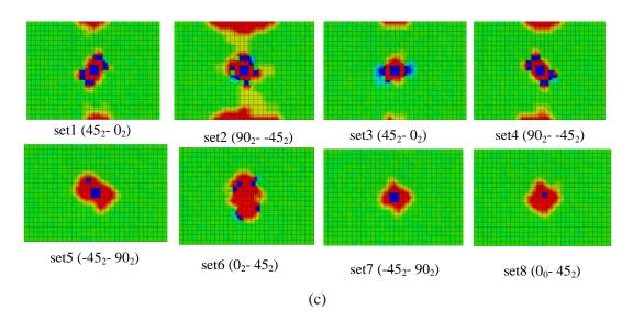
Figure 12. Matrices cracking profiles that were obtained from numerical simulation for various layers at impact energy 35 J for carbon fiber/epoxy at different layups (a)(A  $[90_2, -45_2, 0_2, 45_2]_{2s}$ ), (b)(B  $[0_2, 45_2, -45_2, 90_2]_{2s}$ ), (c)(C  $[45_2, 0_2, 90_2, -45_2]_{2s}$ ).
