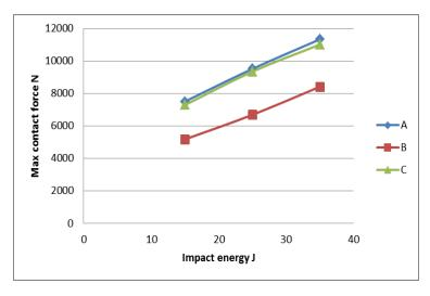
Figure 10. Numerical the maximum impact force vs. impact energy(15, 25, 35) J at equal mass of impactor 5.5 kg (A [90<sub>2</sub>, -45<sub>2</sub>, 0<sub>2</sub>, 45<sub>2</sub>]<sub>2s</sub>, B [0<sub>2</sub>, 45<sub>2</sub>, -45<sub>2</sub>, 90<sub>2</sub>]<sub>2s</sub>, C [45<sub>2</sub>, 0<sub>2</sub>, 90<sub>2</sub>, -45<sub>2</sub>]<sub>2s</sub>).
