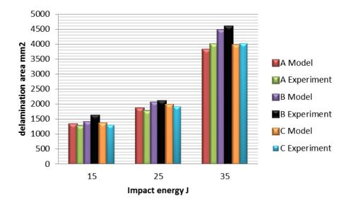
Figure 7. Numerical – Experiment comparison of three different layups in the damage of delamination.
