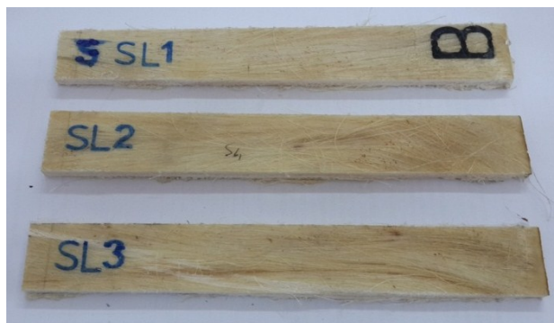
Figure 9. Longitude fibres prototypes of composite materials.
