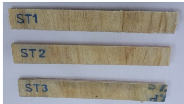
Figure 10. Transverse fibres prototypes of composite materials.
