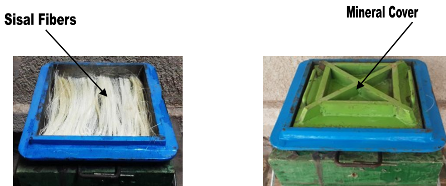
Figure 2. Part of mineral mould using of preparation of specimens.
