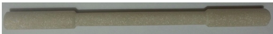
Figure 11. Torsion Fatigue specimen formation of polyester and peel of egg after turning and cutting.
