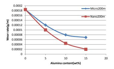
Figure 19. Wear rate at 200m sliding distance for different alumina percentage of micro composite and nano composite subjected to 500g load.
