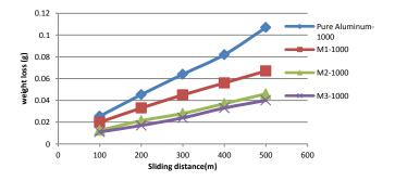
Figure 4. Weight loss for samples with micro alumina additives subjected to 1000g load.
