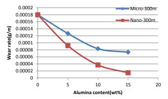
Figure 20. Wear rate at 300m sliding distance for different alumina percentage of micro composite and nano composite subjected to 500g load.
