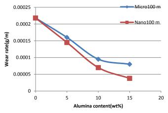
Figure 18. Wear rate at 100m sliding distance for different alumina percentage of micro composite and nano composite subjected to 500g load.
