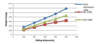
Figure 11. Weight loss for samples subjected to 1500g load, 5wt % micro-alumina M1, 5wt % Nano-alumina N1 and pure aluminum.
