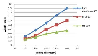
Figure 9. Weight loss for samples subjected to 500g load, 5wt % micro-alumina M1, 5wt %Nanoalumina N1 and pure aluminum.
