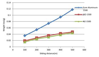
Figure 14. Weight loss for samples subjected to 1500g load, 10wt % micro-alumina M2, 10wt % Nano-alumina N2 and pure aluminum.
