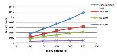
Figure 8. Weight loss for samples with Nano-alumina additives subjected to 1500g load.
