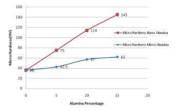
Figure 2. Microhardness results for samples in case of micro composites and nano composites.
