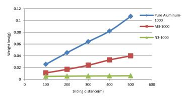
Figure 16. Weight loss for samples subjected to 1000g load, 15wt % micro-alumina M3, 15wt % Nano-alumina N3 and pure aluminum.
