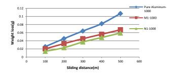
Figure 10. Weight loss for samples subjected to 1000g load, 5wt % micro-alumina M1, 5wt% Nanoalumina N1 and pure aluminum.
