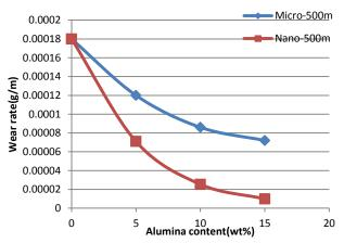
Figure 22. Wear rate at 500m sliding distance for different alumina percentage of micro composite and nano composite subjected to 500g load.
