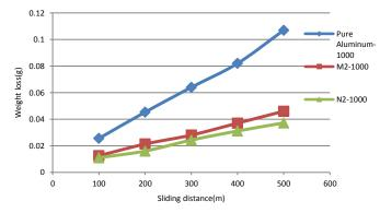
Figure 13. Weight loss for samples subjected to 1000g load, 10wt % micro-alumina M2, 10wt % Nanoalumina N2 and pure aluminum.
