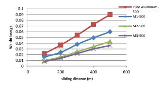
Figure 3. Weight loss for samples with micro alumina additives subjected to 500g load.
