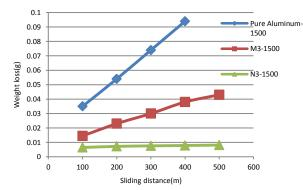
Figure 17. Weight loss for samples subjected to 1500g load, 15wt % micro-alumina M3, 15wt % Nano-alumina N3 and pure aluminum.
