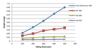
Figure 6. Weight loss for samples with Nano-alumina additives subjected to 500g load.
