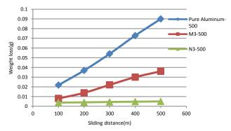
Figure 15. Weight loss for samples subjected to 500g load, 15wt % micro-alumina M3, 15wt% Nanoalumina N3 and pure aluminum.
