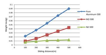
Figure 12. Weight loss for samples subjected to 500g load, 10wt % micro-alumina M2, 10wt% Nanoalumina N2 and pure aluminum.
