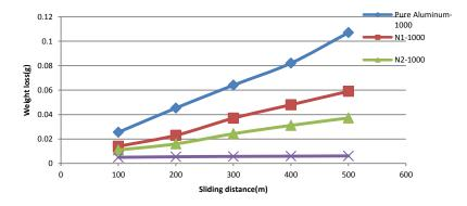
Figure 7. Weight loss for samples with Nano-alumina additives subjected to 1000g load.
