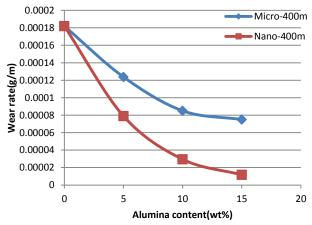
Figure 21. Wear rate at 400m sliding distance for different alumina percentage of micro composite and nano composite subjected to 500g load.
