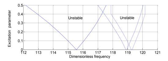
Figure 6. Comparison between the present and the "exact" solution, second mode clamped-pinned pipe  $\gamma=0$ , Uo=2. ( — ) present and "exact" for  $\beta=0$ , (--)"exact" for  $\beta=0.45$ , (-·) "exact" for  $\beta=0.9$ .
