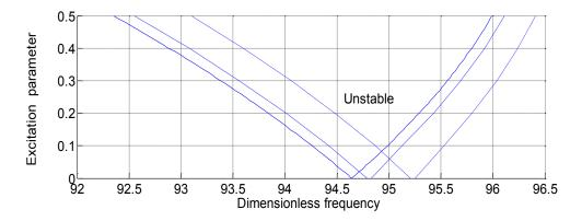
Figure 4. Comparison between the present and the "exact" solution, second mode clamped-pinned pipe  $\gamma=0$ , Uo=2. (-) present and "exact" for  $\beta=0$ , (-)"exact" for  $\beta=0.45$ , (-) "exact" for  $\beta=0.9$ .
