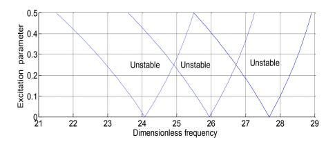
Figure 11. Effect  $\gamma$  on the principal instability regions for the first mode for clamped-pinned pipe  $(-)\gamma=0, (-)\gamma=0.2, (-)\gamma=4.$
