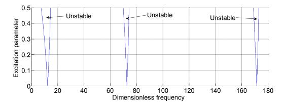
Figure 7. The principal instability regions for the lowest three modes for pinned-pinned pipe.  $\gamma = 2$ , Uo=2.
