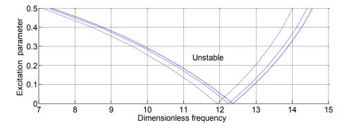
Figure 1. Comparison between the present and the "exact" solution, first mode pinned-pinned pipe.  $\gamma=0$ , Uo=2. (-) present and "exact" for  $\beta=0$ , (-)"exact" for  $\beta=0.45$ , (-) "exact" for  $\beta=0.9$ .
