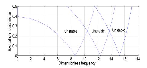
Figure 10. Effect  $\gamma$  on the principal instability regions for the first mode pinned-pinned pipe  $(-) \gamma=0, (-) \gamma=2, (-) \gamma=4.$
