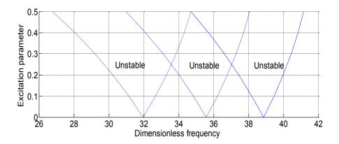
Figure 12. Effect  $\gamma$  on the principal instability regions for the first mode for clamped-clamped pipe  $(-) \gamma=0, (-) \gamma=0.2, (-) \gamma=4.$
