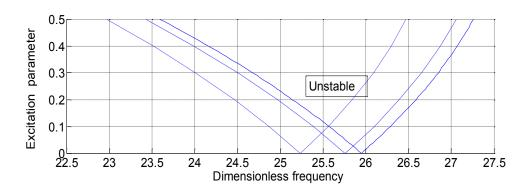
Figure 3. Comparison between the present and the "exact" solution, first mode clamped-pinned pipe.  $\gamma=0,Uo=2.(-)$  present and "exact" for  $\beta=0,(-)$ "exact" for  $\beta=0.45,(-)$  "exact" for  $\beta=0.9$
