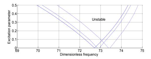
Figure 2. Comparison between the present and the "exact" solution, second mode pinned-pinned pipe  $\gamma=0$ , Uo=2. ( — ) present and "exact" for  $\beta=0$ , (--)"exact" for  $\beta=0.45$ , (-·) "exact" for  $\beta=0.9$ .
