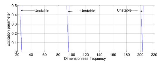
Figure 8. The principal instability regions for the lowest three modes for clamped-pinned pipe,  $\gamma=2, Uo=2$ .
