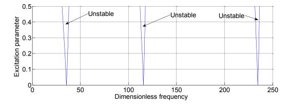
Figure 9. The principal instability regions for the lowest three modes for clamped-clamped pipe,  $\gamma=2, Uo=2.$
