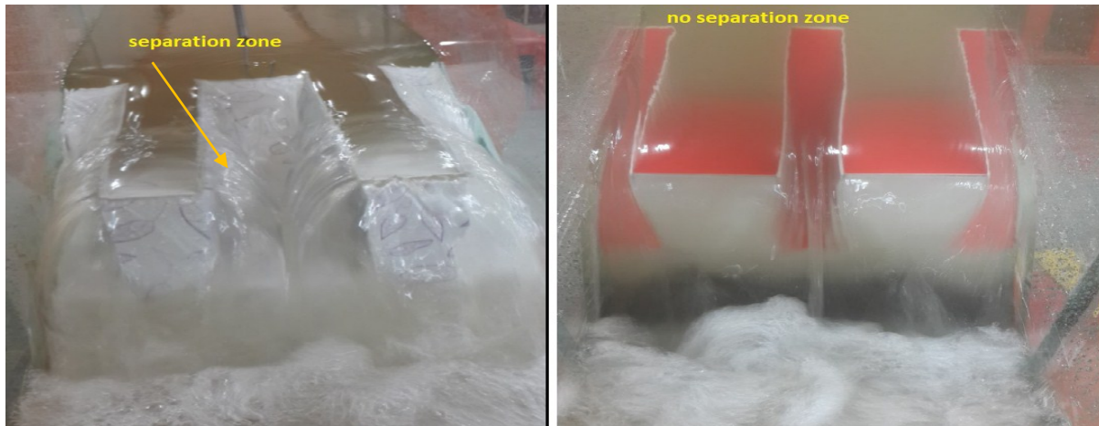
Figure 5. Effects of key width on separation zone at H/P=0.27 over PKW of (a) W_i/W_o = 0.5 (model W0.5), and (b) W_i/W_o = 2 (model W2).
