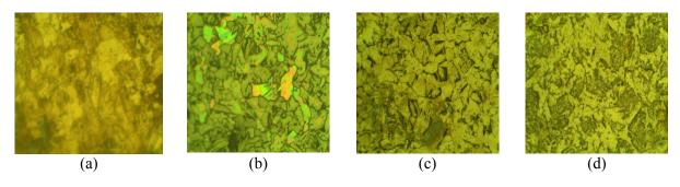
Figure 4. Microstructural examination of (a) as-received sample (b) 25% PE (c) 35% PE (d) 45% PE (at 100x).
