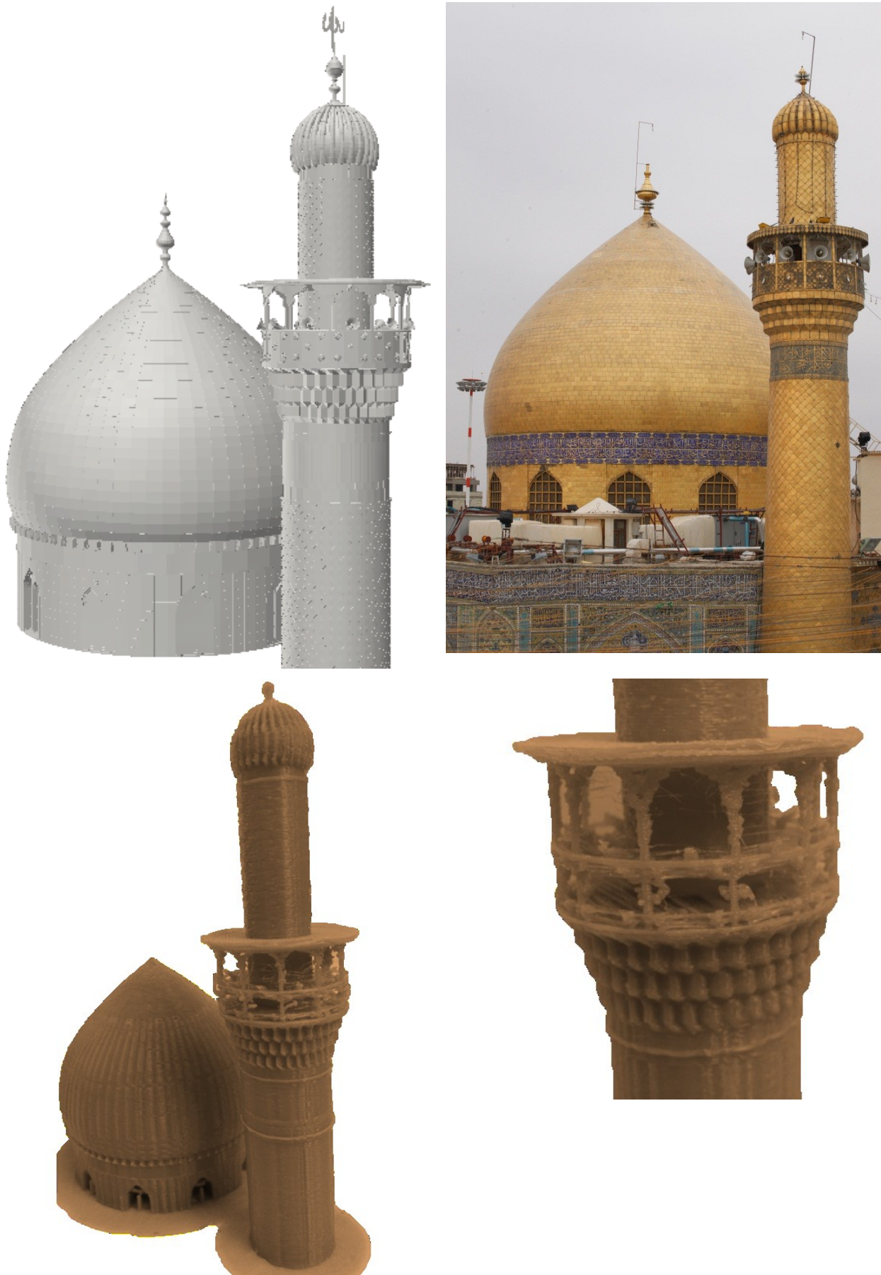
Figure 4. 3D model and 3D print of the golden dome and the golden minaret of the Holy Shrine of Imam Ali bin abi Talib (peace be upon him).
