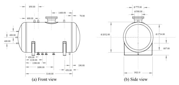
Figure 7. Detailed dimensions of vessel model.
