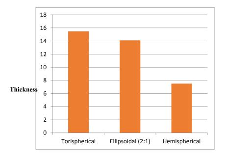
Figure 8. Design thickness of the three head types.
