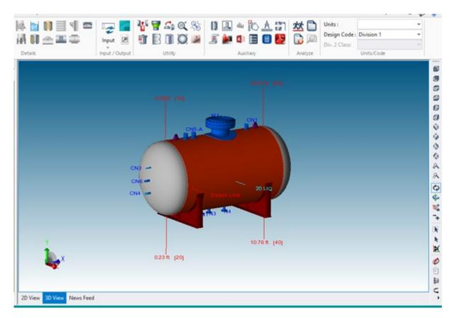
Figure 5. PV Elite wizard window and model building.
