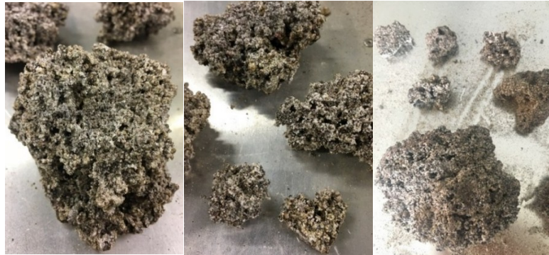
Figure 3. Agglomeration of silica sand particles.
