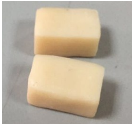
Figure 2. Compression specimen according ASTM 1621.
