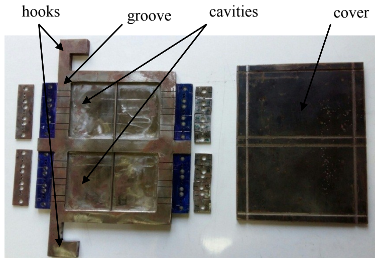
Figure 4. Mold for fatigue test specimens.
