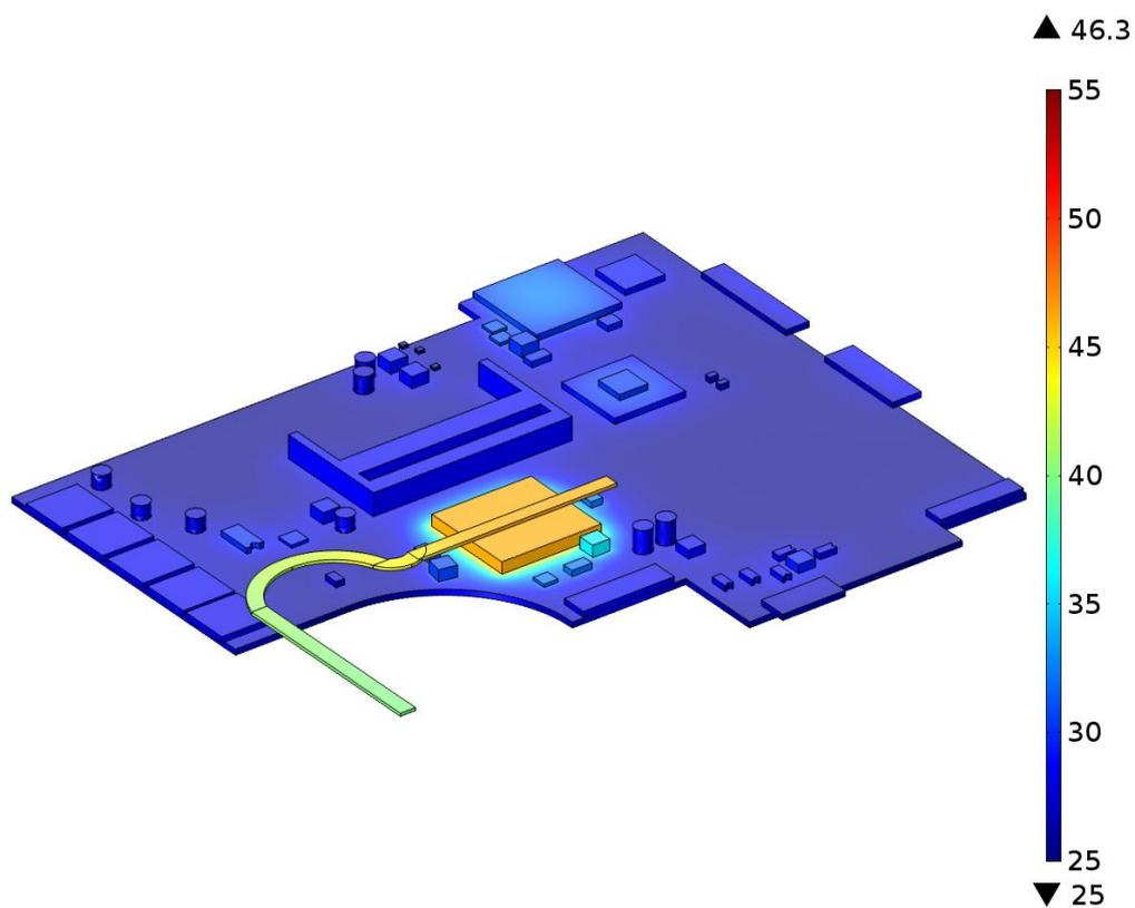
Figure 5. Temperature distribution in the laptop mother board [°C] during operating in the case of fan failed.
