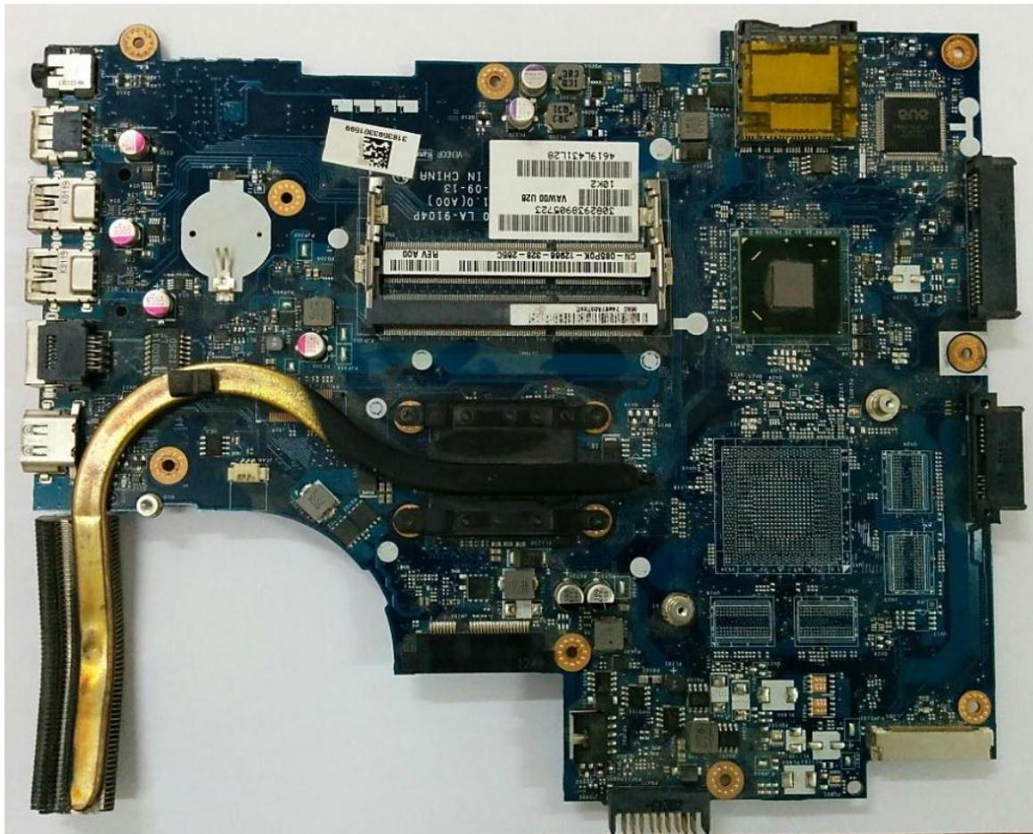
(a) *hp*<sup>®</sup> motherboard with thermal management system (heat pipe).
