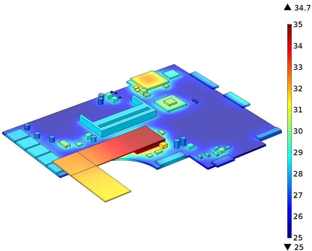
Figure 8. Temperature distribution in the laptop mother board [°C] during operating with new suggested thermal management system (flat plate of copper material coated with graphene and without use of fan).
