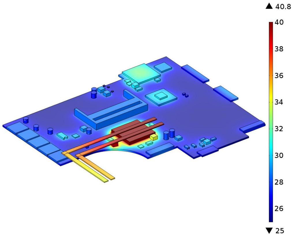
Figure 7. Temperature distribution in the laptop mother board [°C] during operating with new suggested thermal management system (two copper heat pipes).
