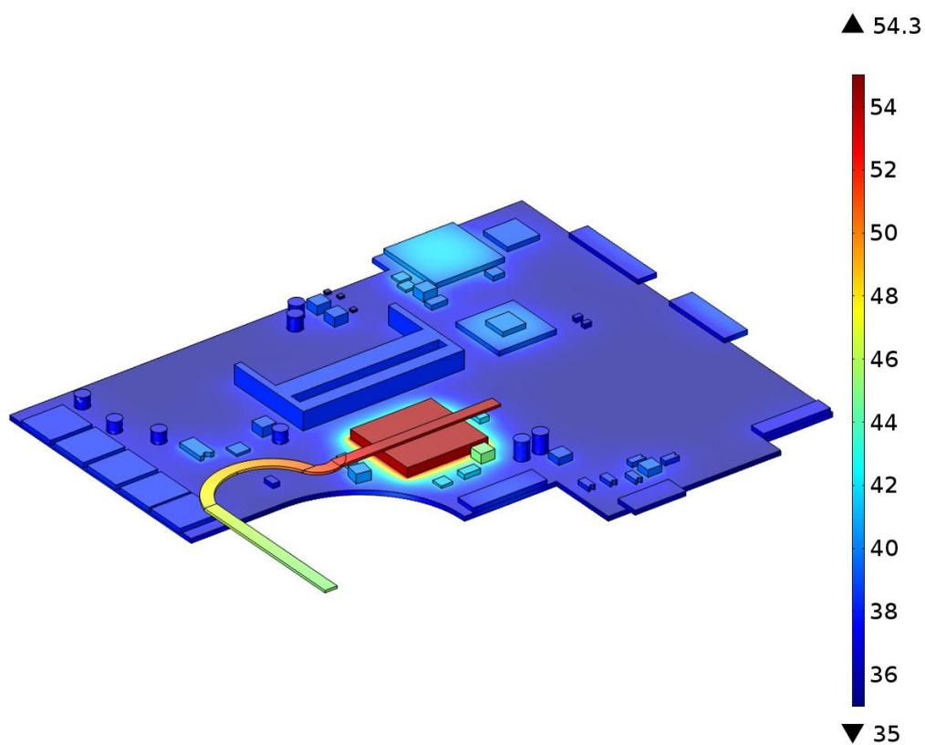
Figure 6. Temperature distribution in the laptop mother board [°C] during operating at ambient temperature of 35 °C.
