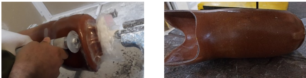
Figure 9. Socket is removed from the positive mold.
