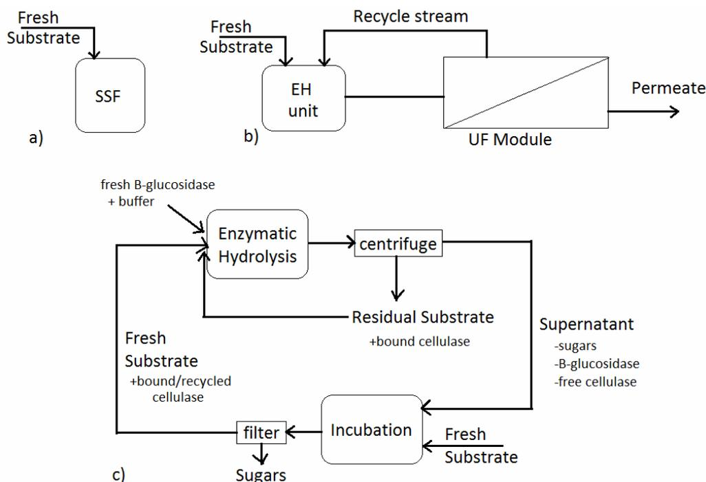
Figure 5. Plausible ways of recycling enzymes: (a) fed-batch simultaneous saccharification and fermentation (SSF); (b) continuous ultra filtration (UF) and (c) recycling of free cellulose from hydrolysis supernatant
