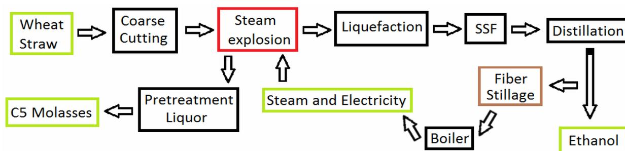
Figure 2. Process flow diagram for IBUS bioethanol production process from wheat straw
