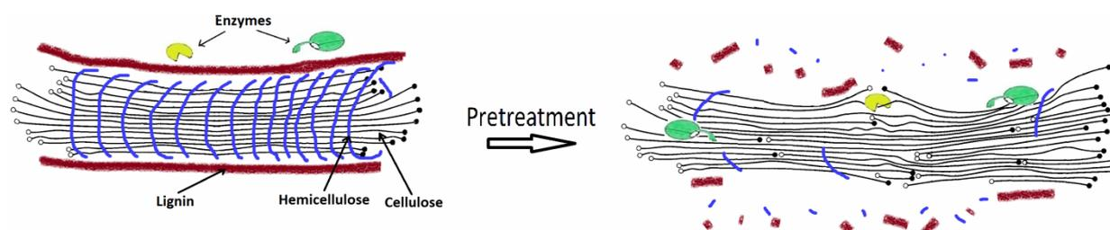
Figure 1. The main goal of pretreatment is to increase the accessibility of cellulose to cellulolytic enzymes in subsequent enzymatic hydrolysis stage
