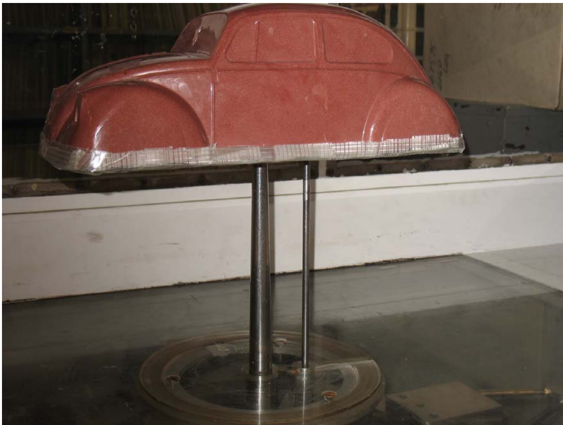
Figure 3. (1:10) scaled car model in the wind chamber of the closed circuit wind tunnel Note: The body is made of clay-like material.
