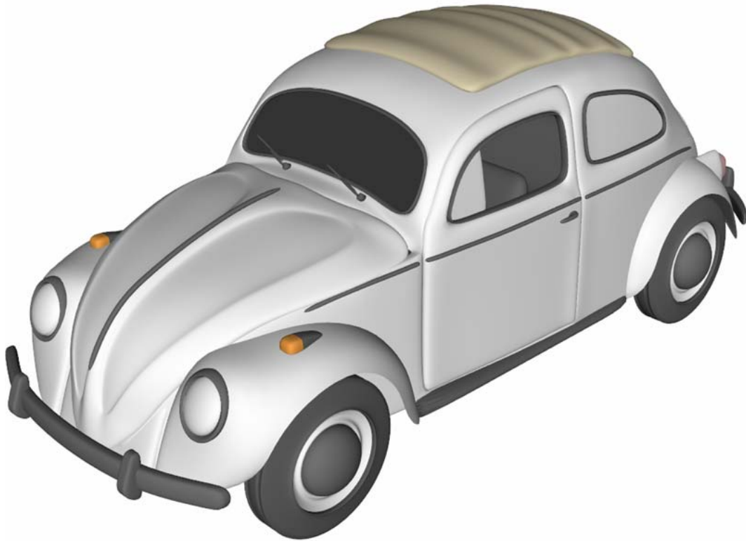
Figure 2. Full scale car CAD model used to replicate air flow behaviour of an actual car Note: See Figure 1 for a picture of the real car in question.
