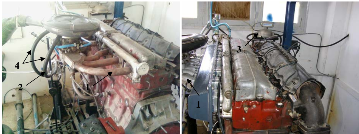
(a) Optimized intake manifold
