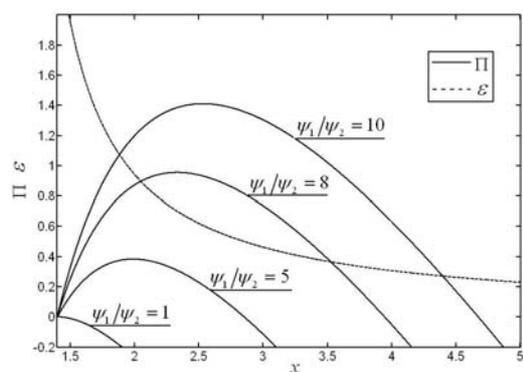
Figure 6. Dimensionless profit rate and the COP characteristic for Brayton cycle
