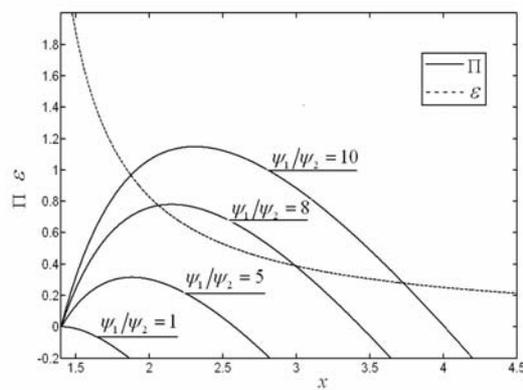
Figure 4. Dimensionless profit rate and the COP characteristic for Diesel cycle
