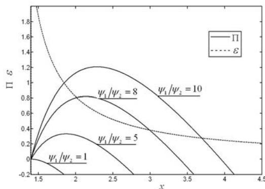
Figure 5. Dimensionless profit rate and the COP characteristic for Dual cycle
