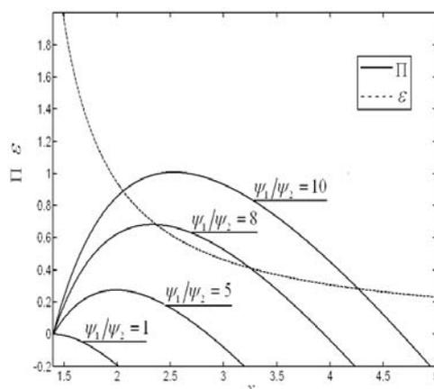
Figure 2. Dimensionless profit rate and the COP characteristic for Otto cycle
