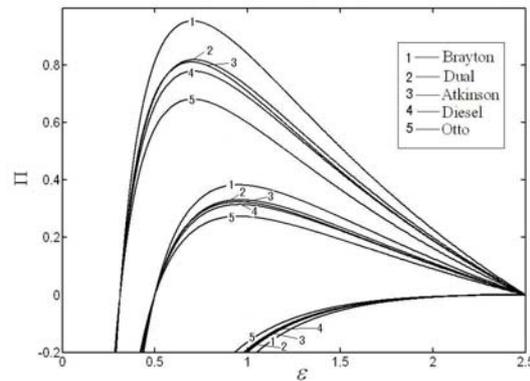
Figure 7. Dimensionless profit rate versus the COP characteristic for five cycles
