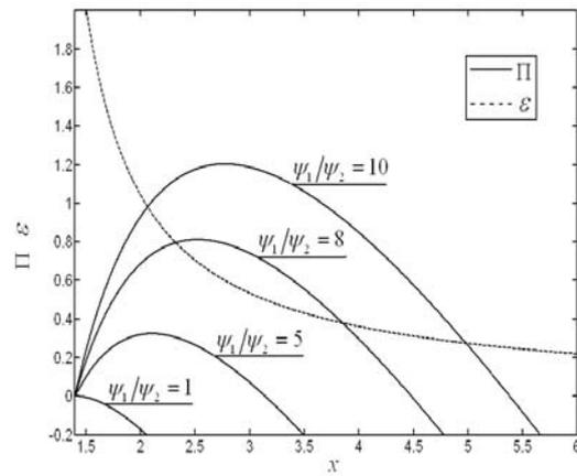
Figure 3. Dimensionless profit rate and the COP characteristic for Atkinson cycle
