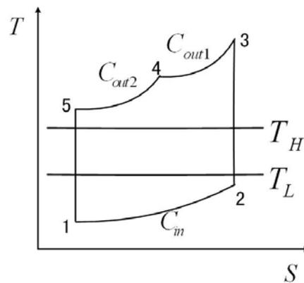
Figure 1. T-s diagram for universal endoreversible cycle model
