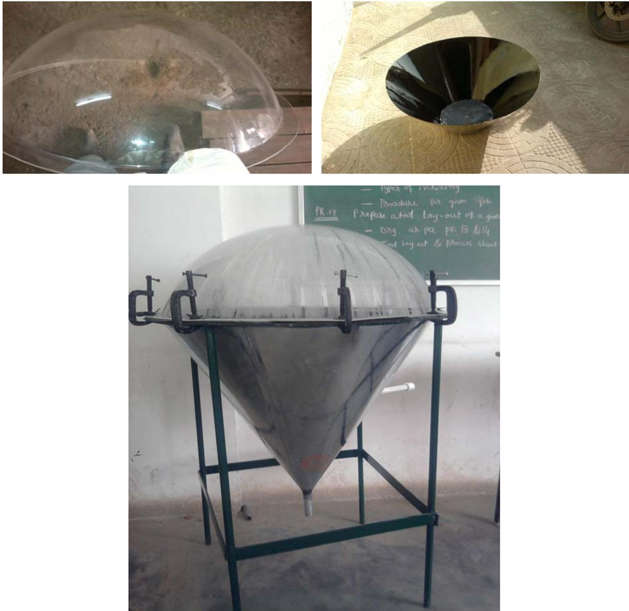
Figure 2. Components as well as complete fabrication of hemispherical solar still
